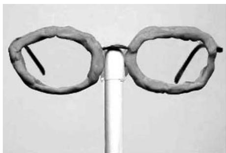
**Figure 2** Tac 'N Stik<sup>®</sup> reusable adhesive around the edges of the eyeglasses used to prevent unmasking.
